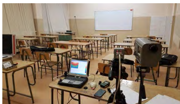
Fig. 7. Measurement equipment for UGR evaluation
